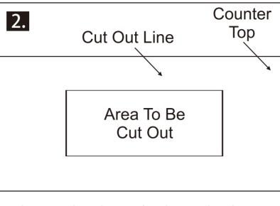
NOTE: BEFORE CUTTING, DOUBLE-CHECK THE MEASUREMENTS OF YOUR TRACED LINE ARE ACCURATE TO THE SINK DIMENSIONS
