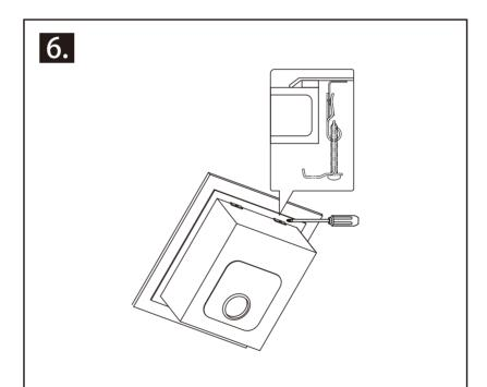
Tighten the fixing clips screws with a hand
