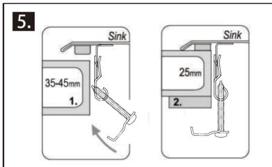
The supplied fixing clips are designed for 35-45mm thick counter tops. If your counter top is thinner, use wood spacers to secure the clips.
