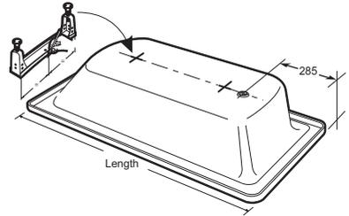
1. Before installation set out the pipe work for the bath and ensure it is aligned with the waste.
