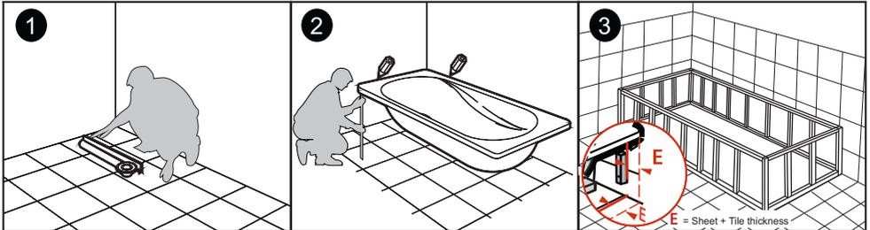
1. Find the desired height of the bath on the wall. A minimum clearance of 10mm is required under the floor of the bath to allow free flexing of the entire bottom of the bath.
