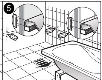
4. Place in position and use the adjusting screws to ensure the bath is completely level. Make sure that the underside of the bath is clear of any obstructions.
