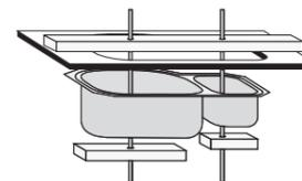
Above shows how threaded rod and timber bearers may be used to clamp the sink in place while fastening to the counter / benchtop using methods B and C.
