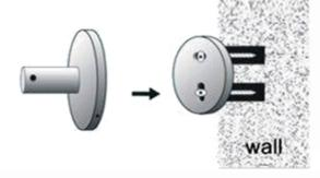
Put the base of bathroom accessory cover on the fixing blocks.
