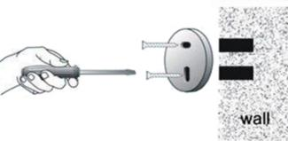
3.Put fixing block cover on the holes and fix firmly by expansion screws.
