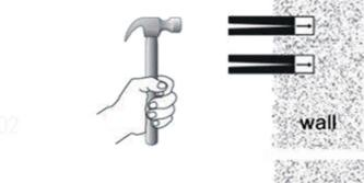
2. Put the expansion plugs into the wall by hammer.
