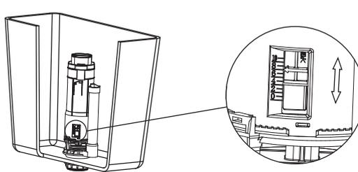
The full flush volume can be adjusted by changing the residual water level in the cistern. Move the adjuster DOWN to increase the volume. Move the adjuster UP to decrease the volume.
