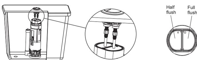
Button rods must be just clear of the valve pads
