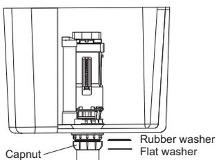
Capnut must be hand tightened to correctly seal flush pipe
