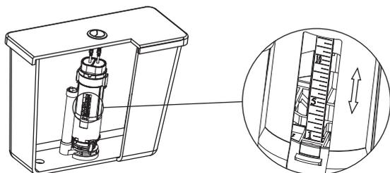
Half flush volume can be adjusted by moving the side float up or down. Moving the float DOWN increases the half flush. Moving the float UP decreases the half flush
