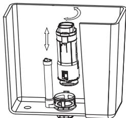
Valve may be removed for service - twist to unlock
