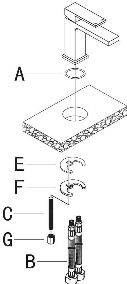
Braided nylon flexible hoses must be inspected every 12 months for warning signs of failure including bulging, rust spots, wear, moisture, snapped threads, kinking, water staining, general corrosion or discolouration. Mixer tails showing any signs of the above mentioned warning signs must be replaced immediately.
