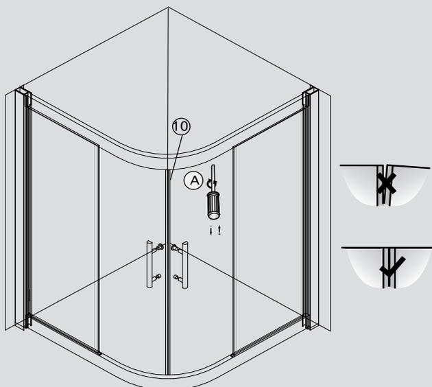
Adjust the sliding doors(4) using the screws located on the bottom of top roller assemblies(13). Adjust rollers so that the sliding doors (4) are parallel to the fixed panels(3) and parallel to each other. Note: Do not overtighten top rollers as this will cause the bottom rollers to jamb and or break.
