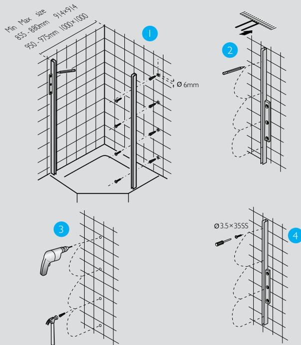
1 Measure your shower base/shower area. The measurement to the outside edge of the of the wall jambs(1) should be somewhere within the min and max size of the screen.
