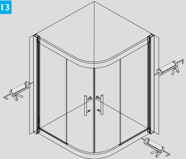
Apply silicone sealer around all external joints of shower screen and **allow 24 hours for silicone to set.**
