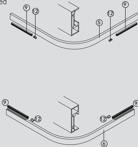
Insert fixed panel end block(12) first then short fixed panel seal(9) into slot on both bottom and top rails(5)(6). (Usually comes preinstalled in top and bottom rail.)
