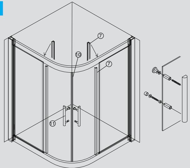
Gently knock the sealing strips(7) onto the fixed panels and doors. Attach the door handles(11) to the sliding doors making sure there is a washer between the glass and the handle. Gently knock the magnetic sealing strip(10) onto the sliding doors.
