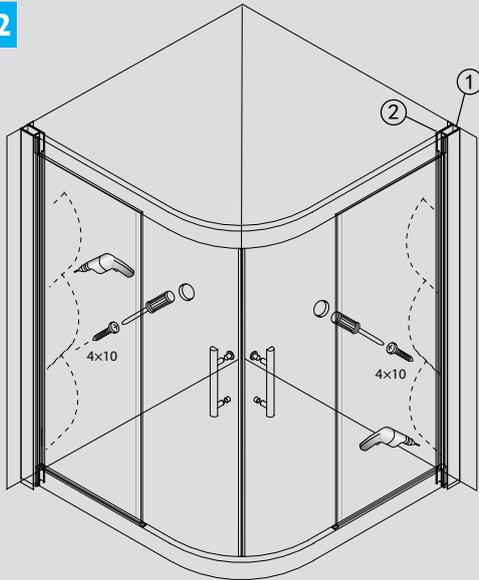
Drill 4 equally spaced holes on the inside of the screen. Fix off wall jambs(1) to the fixed panel extrusion(2) using the screws supplied. Cap all screws.
