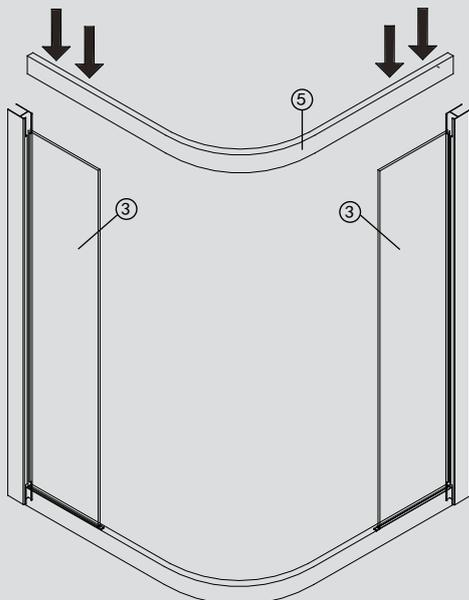
Push fixed panels(3) into seal that is located in the top rail(5). Make sure that the panel is firmly up against the fixed panel block(12) and fully inserted into the short seals(9). Hint-Wet the edge of glass and seal to make it easier to insert panel.
