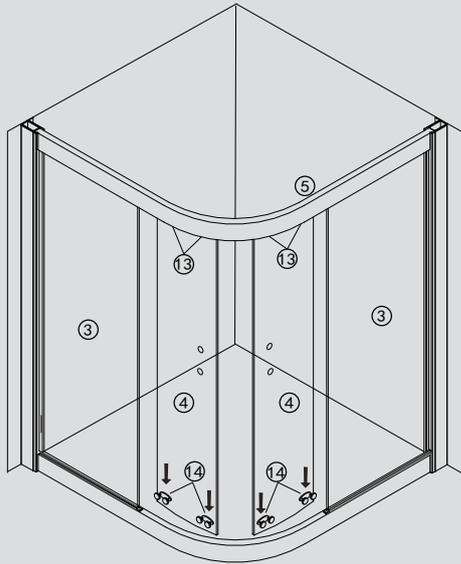
Clip the bottom of the door into the bottom rail(6). The rollers(14) are pressed down to allow the rollers clip to be into the rail.
