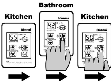
As a safety precaution, if a Kitchen Controller's temperature is set above 50°C, transferring and then returning 'priority' to the Kitchen Controller will result in a default set temperature of 50°C being selected. This is a safety feature.
