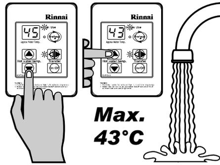
Whilst hot water outlets are open the set temperature may be lowered. However they cannot then be raised above 43°C. In addition transfer of 'priority' between controllers is not possible. These are safety features.
