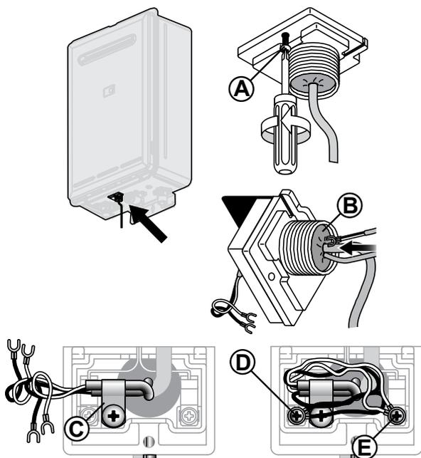
'Ezi connect' cable connector for water heater models:
