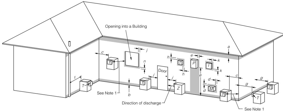
T = Flue terminal    Z = Fan assisted flue appliance only    M = Gas meter    P = Electricity meter or fuse box    I = Mechanical air inlet
