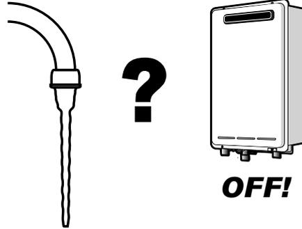
At low water flows, the hot water unit may extinguish without warning. Opening the tap further will restart the appliance.
