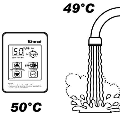
Depending on the weather conditions and the length of the pipe between the hot water unit and the outlet in use, there may be a variation between the temperatures displayed at the water controller(s) and the temperature of the water at the outlet.
