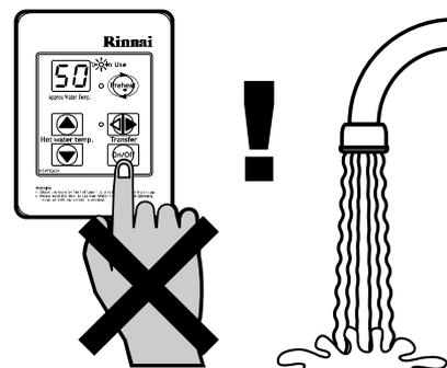
**Do Not** push the On/Off button on any Controller when the 'Red' water heater 'In Use' indicator is illuminated as this will turn off the water heater causing the water to go cold. Someone maybe in the middle of having a shower or filling a bath.
