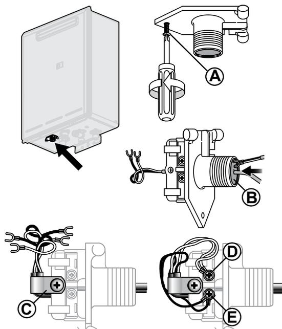
'Ezi connect' cable connector for water heater models:
