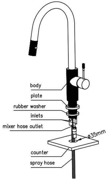
Use a 35mm hole saw cut a hole through the counter. Remove the lock nut, triangle plate, steel washer. Feed spray hose through the hole and position the mixer over the hole.
