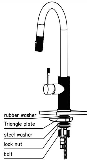
Slide the rubber washer, triangle plate and steel washer and lock nut over spray hose, screw onto thread pipe. Tighten the lock nut firmly and then tighten the 2 bolts on the lock nut firmly as well.
