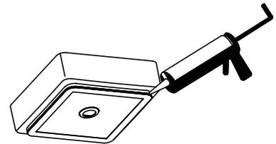
4. Apply silicon glue to the outer base of the basin.
