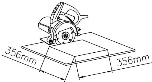
3. We suggest you ask stone vendor or use a professional stone mason to cut desired hole in benchtop.(check measurements twice prior to cutting)
