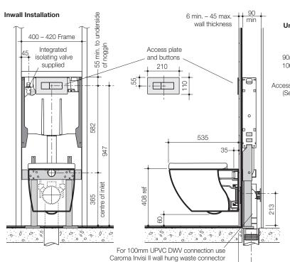
170 max. from finished wall with Invisi II WH pan connector
