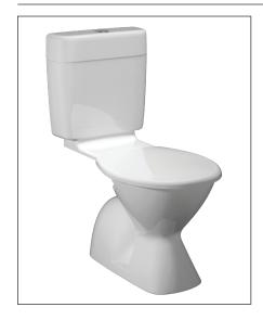
The **Jeda** connector toilet suite with its mid sized cistern is designed for retrofit installations and delivers a 4.5/3 litre dual flush system. Combined with the Stylus Concealed Connector 4.5 litre pan, the Jeda cistern is an integrated system comprising of cistern with high performance outlet valve, Beta seat and flush fitting connection plate, which conceals the flush pipe and water connection.
