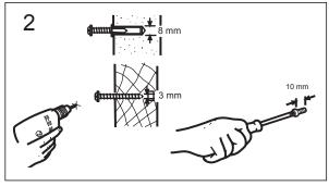
In masonry, drill 8mm diameter holes and insert the plugs provided. In timber, drill 3mm diameter pilot holes. Install the fixing screws leaving the heads protruding by approximately 10mm from the wall.
