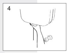
Connect the flush pipe from the cistern to the urinal. In most cases this pipe will be a special fabrication.
