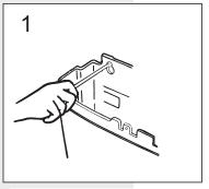
Remove the cistern lid by squeezing the lid on both sides. Hold cistern against wall in the exact position required, ensure that it is level and mark through the mounting holes.
