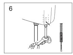
Make sure that the strainer is in place to help prevent damage caused by water borne contaminants. Then fit the water supply pipe using approved fittings.
