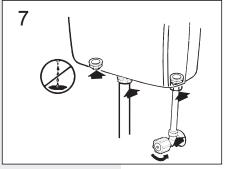
Turn on the water supply and check for leaks at the connection fittings. Allow the cistern to fill and then flush it. Check for leaks at both ends of the flush pipe.
