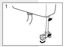
Turn off water supply and if strainer is to be Unclip adjusting cleaned remove connection fittings.
