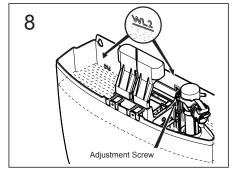
Actuate the Inlet valve at least once to purge any trapped air in the valve.
