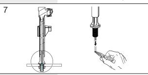
Using pliers carefully remove strainer from the base of the valve.
