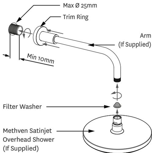
**NOTE: Use plumbers tape or similar on ½" male threaded connection to ensure a reliable seal.**
