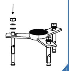
2. put the adapter connect into the triangle.
