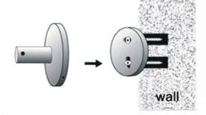
4. Put the base of bathroom accessory cover on the fixing blocks.
