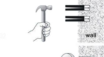
2. Put the expansion plugs into the wall by hammer.
