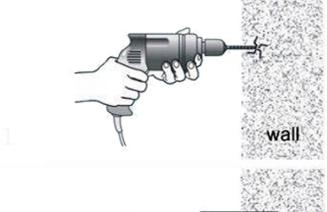
1. Put the fixing blocks (piece) over on the right place on the wall, and stay level, use marking pen through the holes of fixing block to mark out fixing spots on the wall. Then drill holes by electric hand drill with 6mm drilling bit on the spots.
