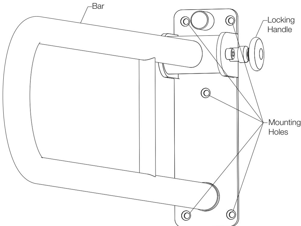
Mark the position of the holes on the wall and remove the Grab Bar.
