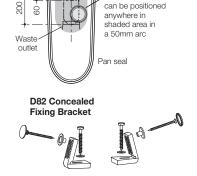
Note: All height dimensions to underside of pan, make allowance for bedding.
