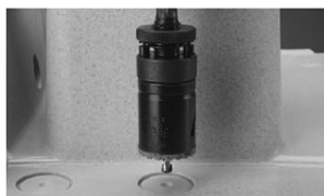
Fig. B - Place the tool on the pre-punched hole.
