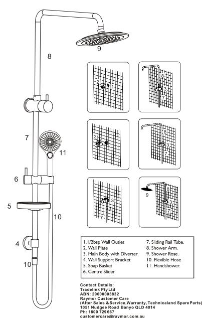
General Note: This product is to be installed by a licensed plumber, installation must comply with AS/NZS 3500 and local plumbing codes.
