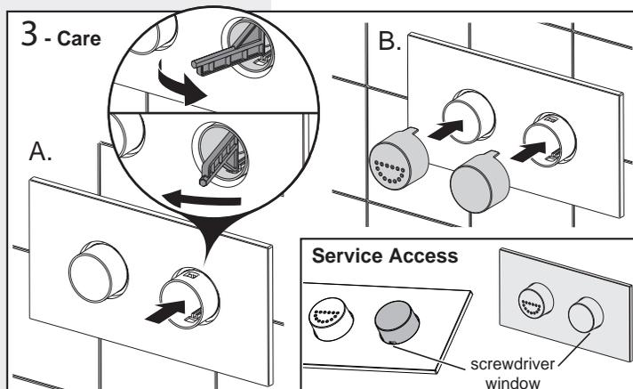
**A.** Depress the full flush button (as provided, without cap) and use the Allen Key to lock the Face Plate to the Mounting Panel top & bottom.
