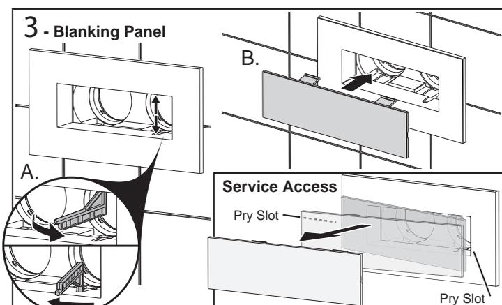
**A.** Allen Key to lock the Face Plate to the Mounting Panel top & bottom.
