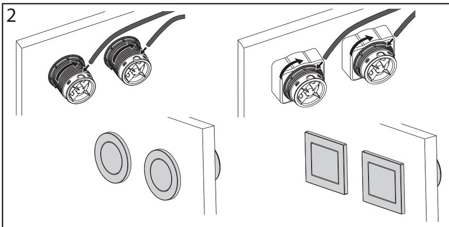
Drill/cut holes according to the specified dimensions above in the desired position.
