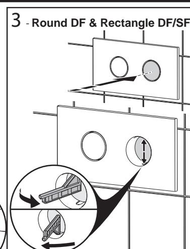
Remove Face Plate from the assembly and set aside. Push the Pneumatic Tubes into the rear of the Mounting Panel assembly ensuring the correct tube is matched with the corresponding button. Use the supplied Allen Key and Mounting Panel Screws to fix the assembly to the Tiling Box or Remote Mounting Box. (Note that the Tiling Box or Remote Mounting Box should be trimmed flush to the wall prior to assembly of the buttons.)
