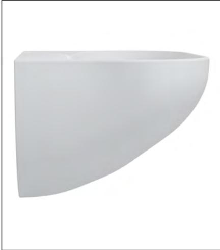
The Clinic 600 basin is an integral trap basin that conceals fittings and features an anti-splash rim. The basin is designed for infection control with easy to clean surfaces. The basin also has a slight gradient on the tap landing to allow effective water run off and a vandal resistant grate. Ideal for wall mounted tapware. This basin is suitable for domestic, commercial and ♿ disabled applications.
