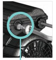
Push the connector into the housing until it 'clicks' into the fixed position.
