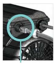
Connect the touch pad cable into the housing, with the alignment shown.
