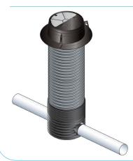
EziPit 600 (MC) is a gravity sewer maintenance chamber with a nominal inside diameter of 600mm. Permitting safe access for cleaning and inspection equipment from the surface but restricting man entry.
